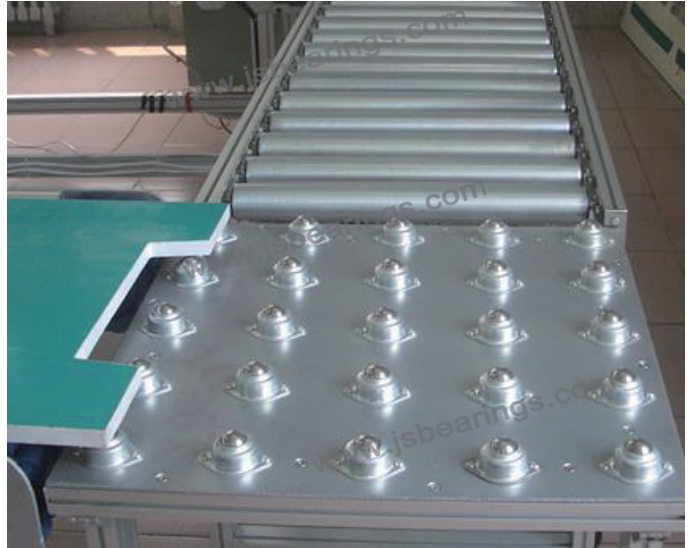
万向球用于车间装配生产线 Used in workshop assembly line
